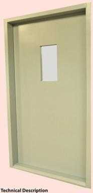
Door frame: 5"x2"(By 16 SWG MS. Sheet) Door Leaf: 1.5" Thick (By 18 SWG MS. Sheet) Shutter infill: Rockwool Paint: Enamel/ Powder Coating/ Epoxy Use: Stair, Lobby, M/C Room etc.
