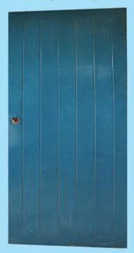
Technical Description Door frame: 5"x2" (By 16 SWG MS, Sheet) Door Leaf: 1.5" Thick (By 18 SWG MS, Sheet) Shutter infill: Rockwool \* Design: Full Vertical Paint: Enamel/ Powder Coating/ Epoxy Use :Home, Office etc.
